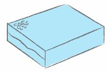
Fish eyes are a pattern of small, under-shrunk spots on the surface of the shrink film that look like shiny flat blisters. They are often caused when some of the film comes in contact with the product too early and cools while the rest of the film is still being heated. To smooth out your surface, have operators turn up the tunnel heat and speed up the conveyor slightly. They may also need to reduce air flow, and use a little less film around the package.
