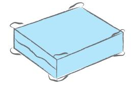
There's several ways to do away with dog-ears those unsightly unshrunk flaps of film that protrude along the seal in the corners. First, increase air evacuation by strategically placed perforations and reduce the bag size. Then, slow down the conveyor while increasing the air velocity and increase the tunnel temp. Redirect the tunnel's air flow to the ends of the package to target the cleanup points.
