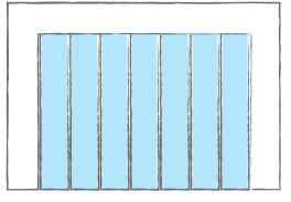
Most tunnels are manufactured with curtains at the entrance and exit of the tunnel. Too often, they are cut off or folded back. This can indicate that the tunnel is not sized appropriately for the packages being run or there are maintenance issues with the tunnel. Curtains are there to maintain consistent heat and should aid in creating consistent, highquality packages.
