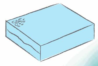
Fish eyes are areas of small, under-shrunk film on the surface of the package. Often appearing in a pattern, these fishy flaws are caused when areas of the film come in contact with the product too early and are cooled while the rest of the film is still being heated. Turn up the tunnel heat and speed up the conveyor slightly. You may also need to reduce air flow, and use a little less film around the package.
