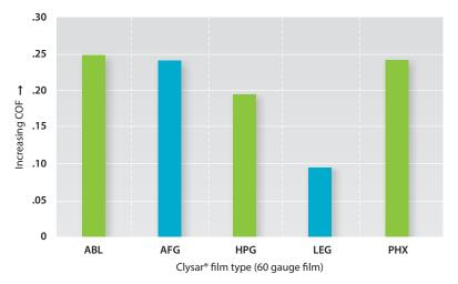
**Coefficient of Friction (COF)** – The ability of the film surface to move against itself or another surface. The higher the coefficient of friction, the more difficult to slip or move (tackier). The lower the coefficient of friction, the easier to slip or move (slipperier).
